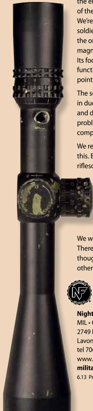
**The hole you see** in this well-used Nightforce 3.5-15 x 50 MIL-SPEC scope at left was made by an enemy 7.62x39 round fired at a U.S. soldier. The bullet completely penetrated the erector tube—the heart of the scope's optical system. We're happy to report that the soldier was not injured, and the only casualty is the scope's magnification ring, frozen on 15x. Its focus, tracking, and all other functions work just fine. It holds point of aim like new.
