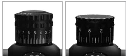
*Nightforce riflescopes equipped with ZeroStop™ and Hi-Speed adjustments can be easily identified by the distinctive domed elevation cap and more closely spaced markings (left, above). Non-ZeroStop™/non-Hi-Speed models have a flat top and greater spacing between markings (right).*
