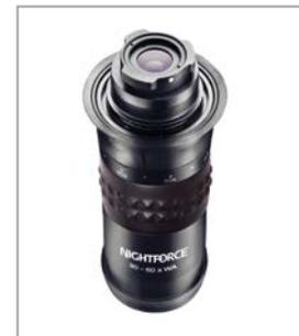
**30x-60x Wide Angle Eyepiece** interchanges with the standard TS-82™ eyepiece and provides a wider field of view. Highly useful for tracking moving and/or multiple targets over a broad expanse. Part No. A275
