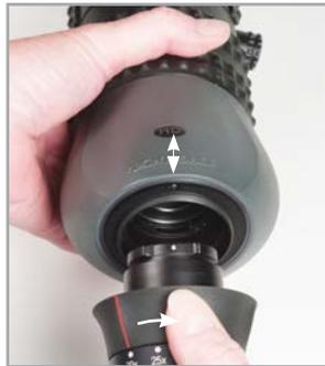
To install the eyepiece, align the white dot of the eye piece with the dot on the scope body. This aligns the bayonet mount of the eyepiece with the proper slots on the spotting scope body. Gently insert the eyepiece into the scope body, and then rotate approximately 1/4 turn clockwise to lock the eyepiece in place. **Important: Do not change or remove the eyepiece in the rain,**
