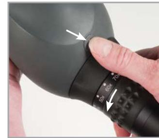
To change the eyepiece, press the Eyepiece Release Button located on the scope body, under the eyepiece. Hold the button down while grasping the scope body securely with one hand. Use your other hand to rotate the eyepiece approximately 1/4 turn counter-clockwise and gently pull it away from the spotting scope body.
